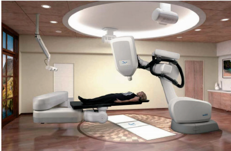
Figure 1: Actual clinical system including the robot arm pointing the 6 MV LINAC to the target. Real-time image guidance based on 6D X-ray imaging (cameras mounted on ceiling, detectors to either side of the treatment couch) provides for frameless radiosurgery applications. The patients is positioned on a robotic patient couch.
